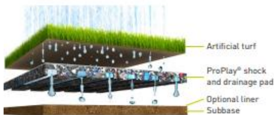
Artificial turf system with ProPlay®-Sport shock and drainage pad
